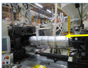
Energy saving of injection molding machine heating cylinder (Left: Close-up of injection molding machine)
