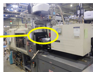
Energy saving of injection molding machine heating cylinder (Left: Close-up of injection molding machine)
