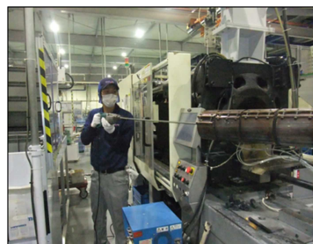
Cleaning of heating cylinder
